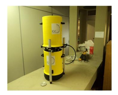
Fig. 2.5 Absolute gravity meter A10-32
