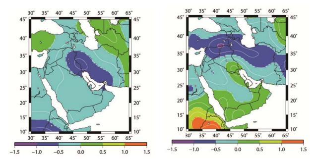
Figure 4: Secular trend (cm/yr) in groundwater during 2003-2012 due to (Left figure) naturally occurring estimated from the CLM4.5 ground water results and (Right figure) Human-made estimated from GRACE data.
