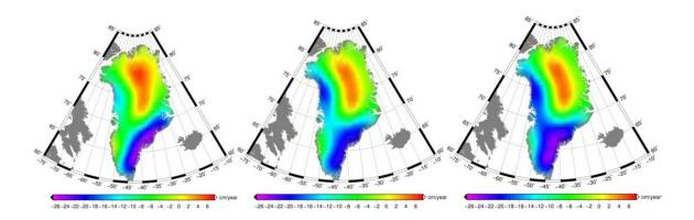
Figure 1: GRACE model estimation of the Greenland Ice mass rate in units of equivalent water height per year (cm/year). The left figure is the averaged rate from February 2003 to December 2007, the figure in the middle is the averaged rate from February 2003 to December 2010, and the right figure is the averaged rate from February 2003 to November 2012.
